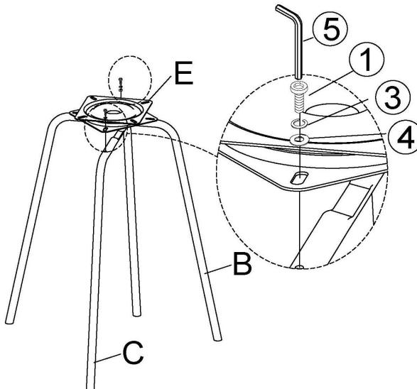
Attach Rotary Turntable(E) to Lower Leg Frame(C) using Bolts(①), Washers(③) and Spring Washers(④) with Allen Wrench(⑤) as shown above.
