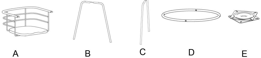
Place the Stool Top(A), Upper Leg Frame(B), Lower Leg Frame(C), Metal Ring(D) and Rotary Turntable(E) onto a clean, non-marring surface.
