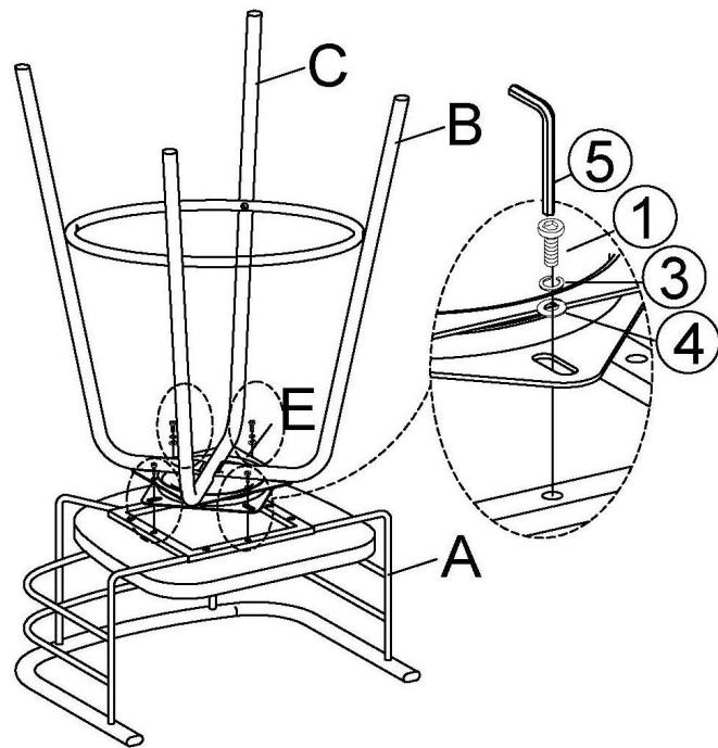
**Attach Upper Leg Frame(B) and Lower Leg Frame(C) to Stool Top(A) using Bolts(①), Washers(③) and Spring Washers(④) with Allen Wrench(⑤) as shown above.**
