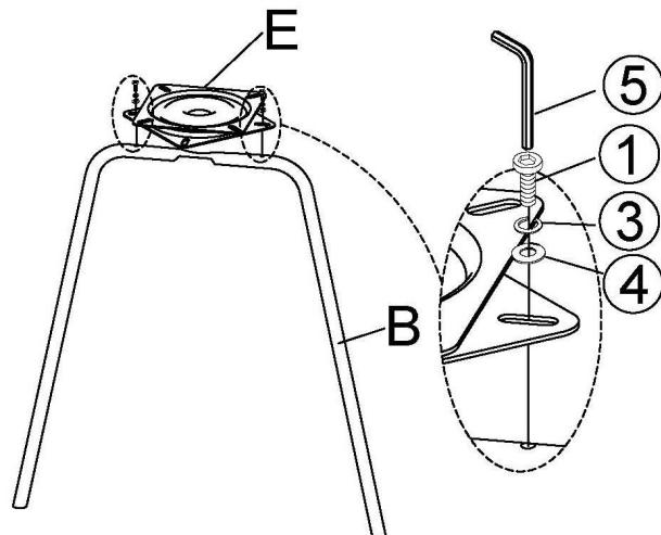
Attach Rotary Turntable(E) to Upper Leg Frame(B) using Bolts(①), Washers(③) and Spring Washers(④) with Allen Wrench(⑤) as shown above.
