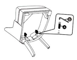
Attach item code A. Making sure to use both washers on each bolt, add the small washer to the bolt firstly then the large washer. Thighten the bolts, initially finger tight.
