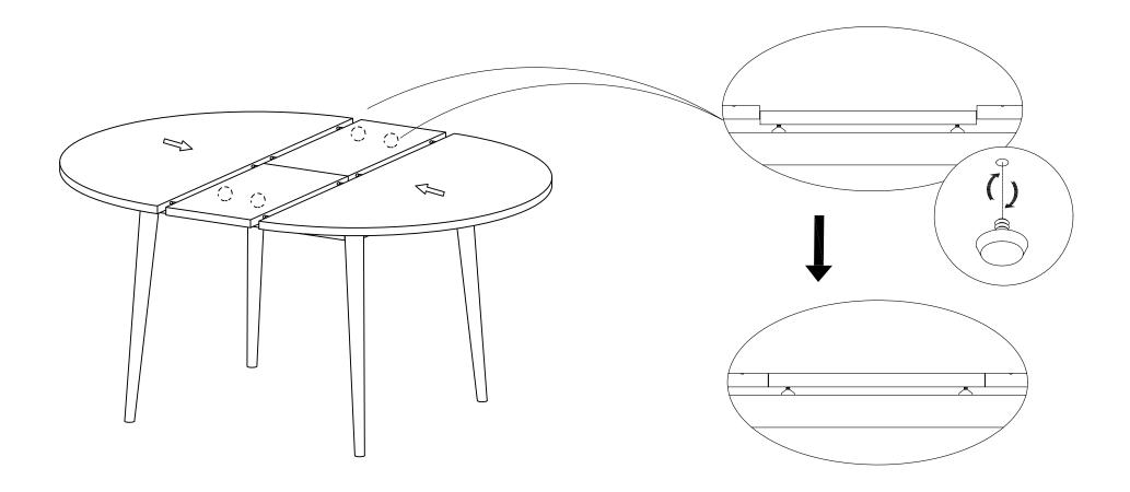
The central panels must be at the same level as the panels on each side.
