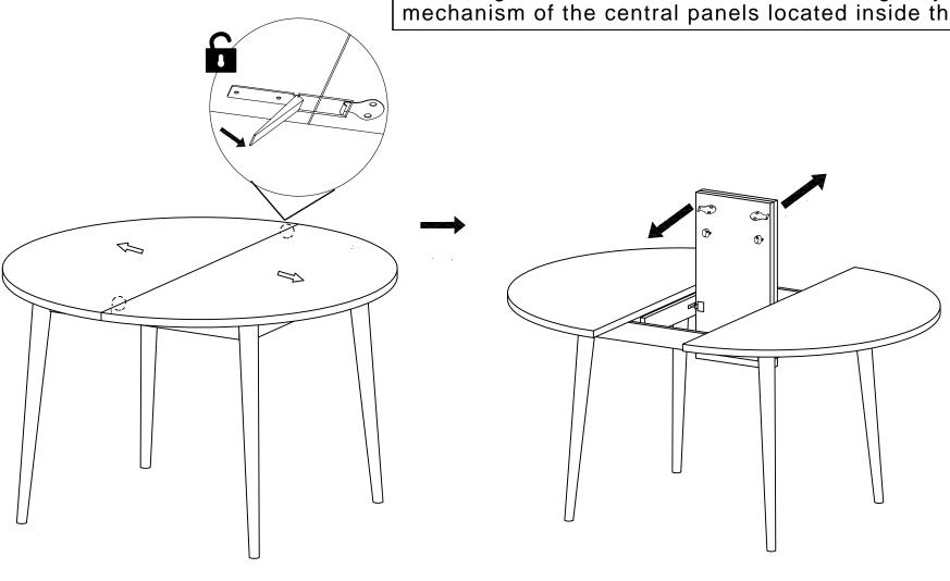
It's important to adjust the height of the central panels by tightening/loosening the screws so that the central panels are aligned with the panels on each side.
