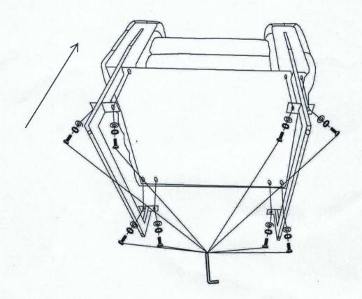
Insert the metal leg into the gap and tighten the hardware with a wrench
