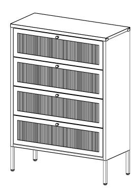
Gaps may appear between the top of the doors and the frame if the item is not on level ground; use the plastic foot cover to level.
